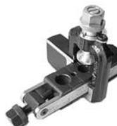
Forms 37° flare to AN standards in steel, stainless steel (including MIL-T 6845), titanium, an other metal tubing. Three rollers in flaring cone roll out 37° flare above die block. Extension on yoke for clamping in vise. Furnished in plastic kit. Wt. 2-1/2 lb.
