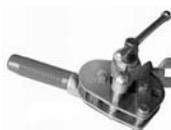
Operates on same principle as Imperial #507-FA but flares 1/8" (primer line) and 3/4" tubing as well. Size: 4"W x 4"D x 8"H. Wt. 2-1/2 lbs. Excellent tool for bench - not for close-quarter work. Not for use on Stainless Steel Tubing.
