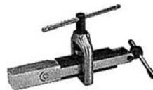
Tool Flares: 1/8", 3/16", 1/4", 5/16", 3/8", and 1/2", O.D. tubing. Forms 37° flares in annealed stainless steel (MIL-T-6845 or AMS-5566), cold drawn stainless steel, and annealed copper, brass, steel or aluminum. Bar has vice extension. Wt.: 3lbs. P/N 12-01166.....
