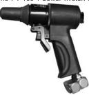
with installation loads of 3500 lbs. or less. All blind rivets from 3/32" dia. up to and including 1/4" dia. CherryMax rivets can be installed with the P-100-1. It utilizes a patented two-valve hydraulic pump actuated by 90 to 130 PSIG air pressure. Unlike most riveters, the P-100-1's collect/jaw assembly remains stationary while the outer sleeve-nosepiece assembly is hydraulically moved, creating sufficient load to install the rivet. Furnished with three nosepieces for 1/4", 1/8", 3/16"
