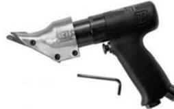
This air-powered shear cuts straight lines or curves up to 180 inches/minute. An ideal shear for any aircraft builder. Cuts up to 18 gauge mild steel. Width of cut: 7/32". Length: 8-1/4". Wt. 2.14 Lbs.
