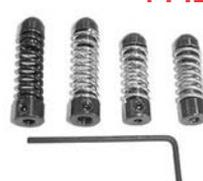
Use when drilling in sheet metal to help eliminate drill breakage & surface marks. Safely keeps drill from going too far through the work. Drill stops have a coiled spring to cushion the drill breakthrough & prevents the drill chuck from marring the work surface. Color coded for easy identification.
