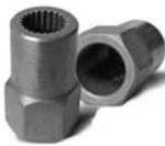
Our Two Step Stud Extractors are the simplest way to remove broken studs and require only 1/8" of the broken stud for removal. Simply tap stud remover on stud or frozen bolt with a hammer or mallet, and then remove stud by attaching a wrench to the hex portion of the remover. Just hammer on and screw out. Built to
