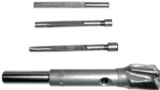
The Spotface Kit tool makes a flat spot for screws. This tool is specifically modified to provide rail cap clearance for use on seat rails. Cutter comes with 1/8", 5/32", 3/16" pilots. P/N 05-04429
