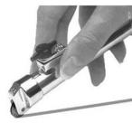
The Beugler tool makes accurate lines consistently, without gravity or pressure, eliminating the need for tape. unique The serrated wheel and wheel head design are the secret to the striper's suc-
