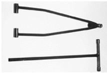
**CESSNA** - This two piece telescoping tow bar fits all Cessnas with 5/8" lugs on nosegear. Overall length 42.5", collapsed 24".
